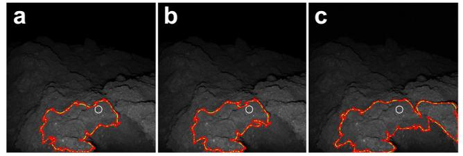
**Figure 8.** The effect of noise on growing a region in the middle of the image. The white, red and yellow outlines represent the starting region from with the growing algorithm started (compare with Figure 5a), rough contour and reference contour. a) Original image, b) additive noise of 10% of the mean pixel value, c) additive noise of 50% of the mean pixel value. Note that the grown region approaches the image boundary on the right in c) which causes a smaller fractal dimension.
