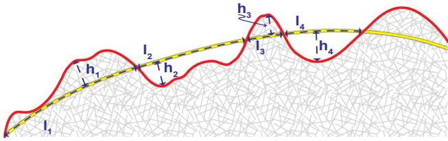
**Figure 4.** Illustration of the derivation of the fractal dimension of a 2-dimensional profile. Shown is the measurement (blue dashed lines) of base length and asperity height of a natural contour (red line). The reference contour is sketched as yellow line.
