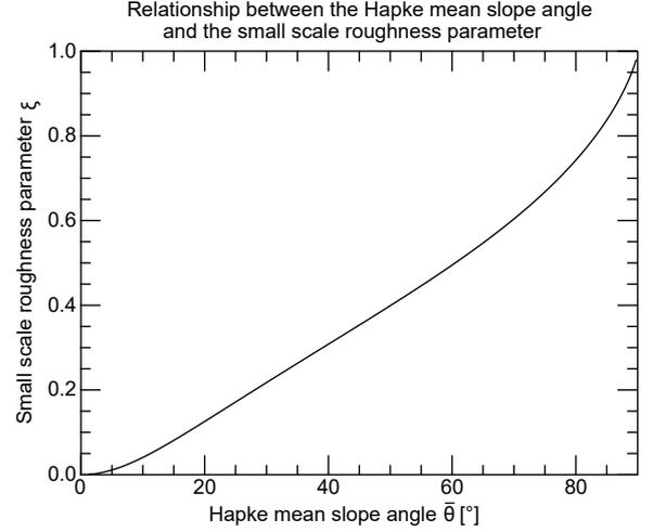
**Figure 3.** Relationship between the Hapke mean slope angle and small scale roughness parameter (Equation 6). The relationship is approximately linear in the regime of most planetary surfaces with  $\xi \approx 0.009 \cdot \bar{\theta}$ .
