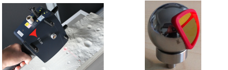
(c) T-Scan for point cloud measurements (d) Laser reflector installed on reflector holder
