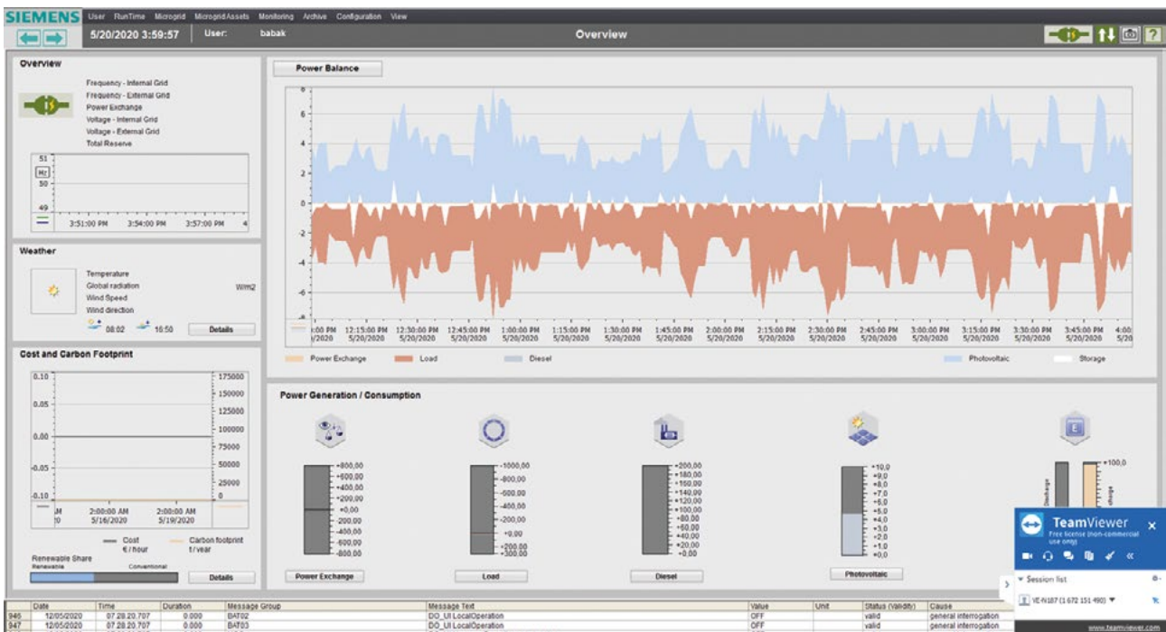
Figure 38: Minigrad Monitoring & Evaluation Data Dashboard – Display of the Siemens Mini-grid Controller Dashboard
