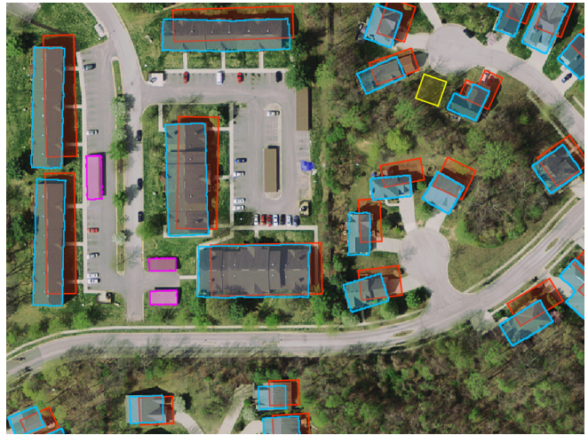
Fig. 4: Alignment result in bloomington22. Noisy OSM annotations are overlaid in red. MapRepair prediction is in cyan. Removed annotations are yellow and segmented buildings are pink.
