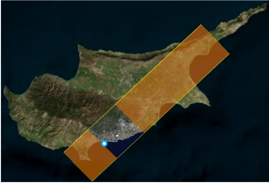
Fig. 1. Footprint of DESIS acquisition over the southern coast of Cyprus (9 th of June 2020), covering most of the island’s southern coast. A sample DESIS quicklook depicted as a true color combination for a single tile including the Amathus harbor is overlaid. The location of the submerged harbor is indicated by a blue circle.
