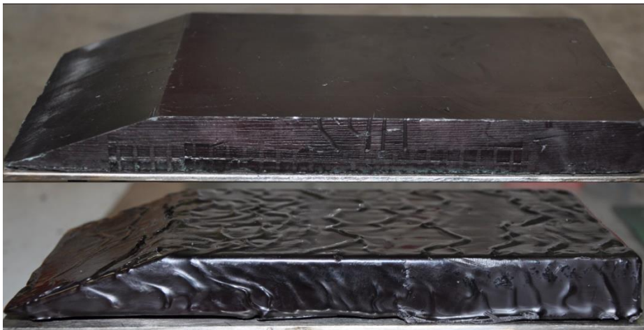
Fig. 1: Fuel slab configuration before (top) and after (bottom) combustion test.
