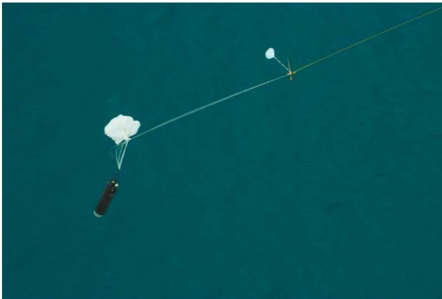
Figure 28: Flight demonstration MAR of Electron first stage test article [29]
