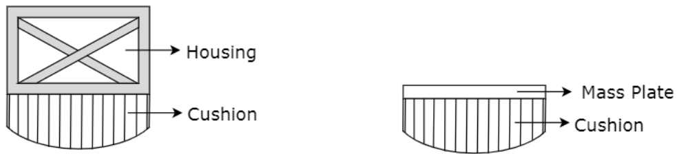
Figure 6: The laboratory set up of the cushion and housing is shown on the left and an equivalent system for correlation is created as shown on the right. The model of the housing is simplified to a mass plate in the FE analysis. The cushion model shown here is of cushion geometry-Model 1.
