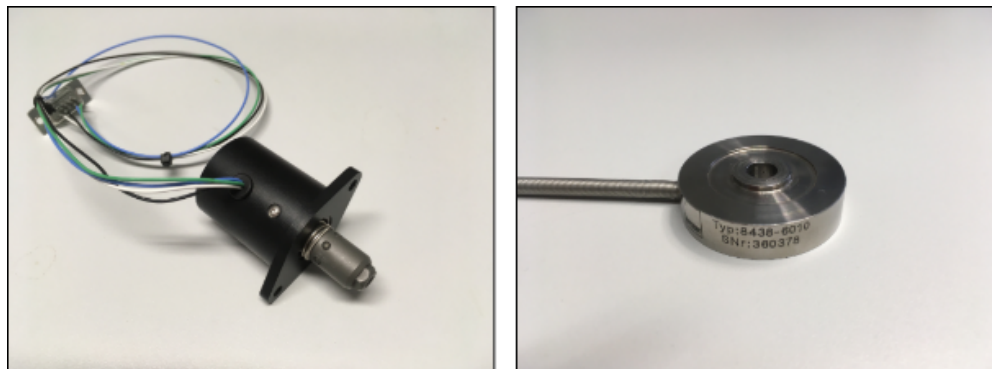
Figure 59: The actual Ejector release mechanism is shown on the left and the load cell is shown on the right.
