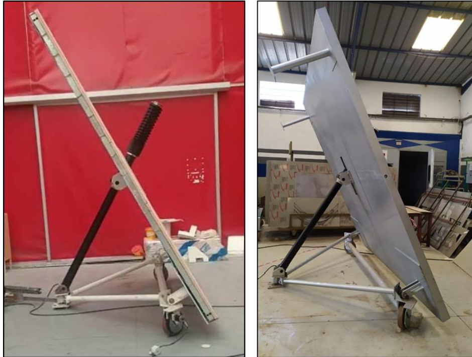
FIGURE 6. Carousel heliostat prototypes of the HelioMaroc project [Jet Energy (left), Aviarail (right)]
