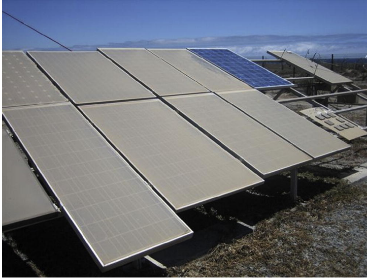
Figure 2.13: Heavily soiled modules on the Gran Canaria Island. A manually cleaned module is visible at the top right corner. [38]
