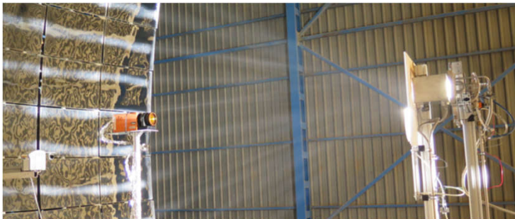
Testing of secondary mirrors in CIEMAT's solar furnace
