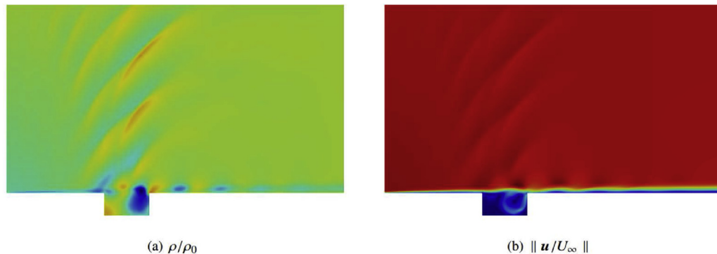
Fig. 31. Plots of the flow results and the decomposition of the Mach 0.8 cavity. (a) The relative density of the flow field displays compressible flow structures and the resulting acoustic wave propagation in the flow domain. (b) The magnitude of the flow velocity indicates the presence of the shear layer mode.
