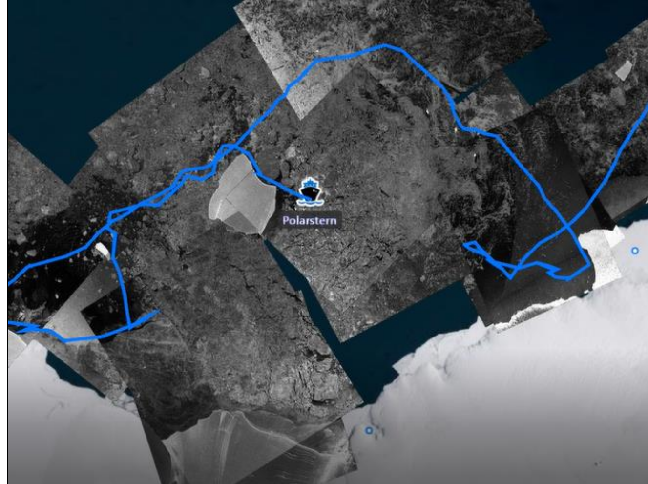
TerraSAR-X Acquisitions delivered in near-real time during AWI Polarstern-Campaign (TerraSAR-X ScanSAR: 17 m Resolution)
