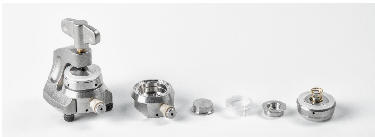
Figure 3.6: ECC-PAT-Core cell with cell holder (left). Consisting of cell base with reference pin, lower plunger, insulation sleeve, upper plunger and lid with PE-seal and spring (from left to right).
