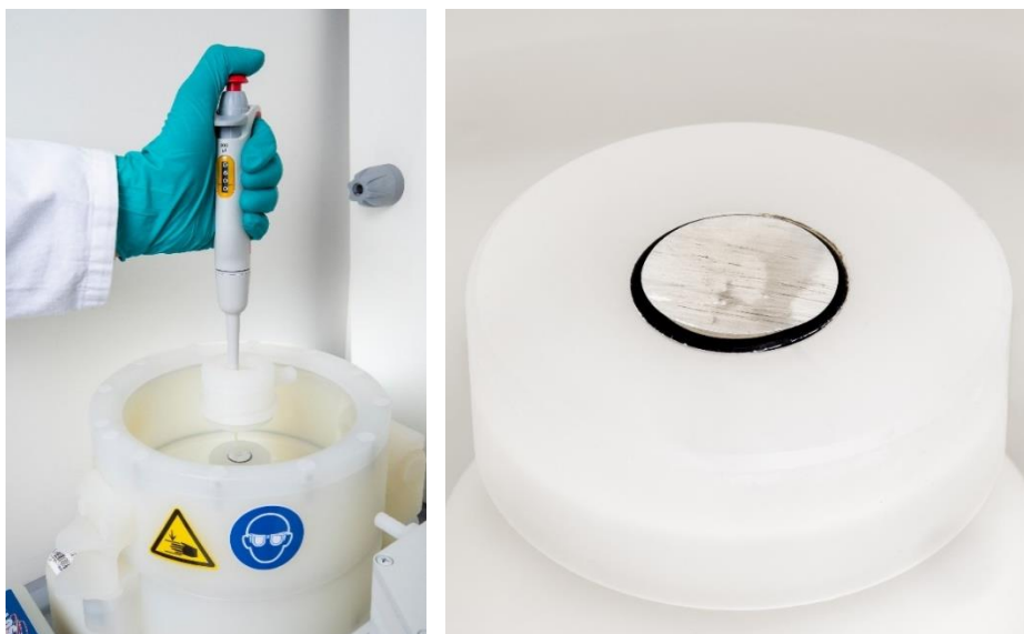
Figure 3.4: Application of coating solution at full spin speed (left) and coated substrate (right).
