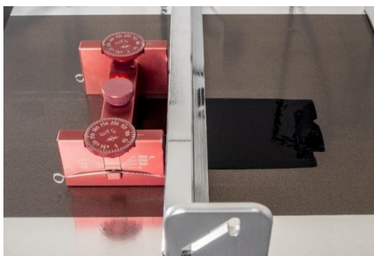
Figure 3.5: Sulfur cathode preparation using doctor blading.
