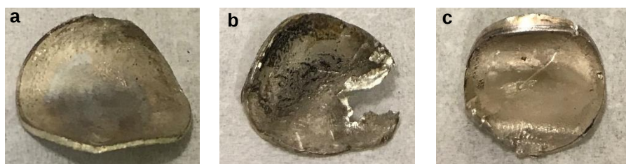
Figure 4.34: Post-mortem images of (a) the uncoated Li anode as well as (b) Li-Nafion/PVDF and (c) Li-SPEEK/PVDF.
