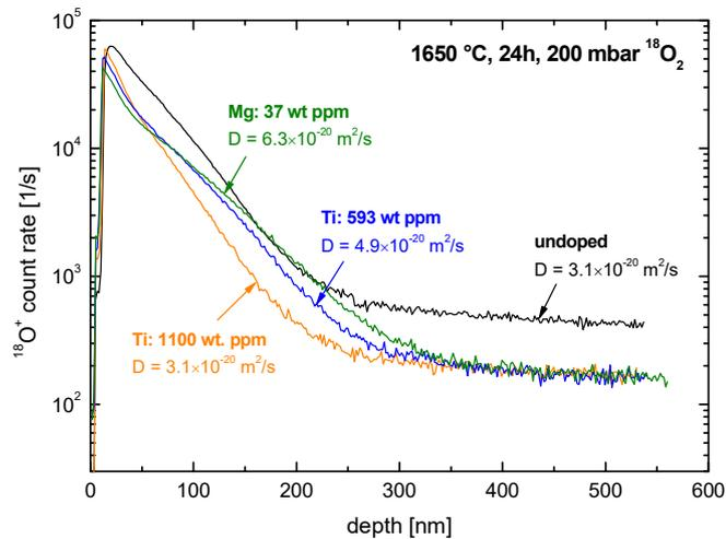
Fig. 2 Comparison of  $^{18}\text{O}$  SIMS depth profiles of four  $\alpha\text{-Al}_2\text{O}_3$  samples (undoped, 593 wt ppm Ti, 1100 wt ppm Ti, 37 wt ppm Mg) which were simultaneously annealed for 24 h at 1650 °C in 200 mbar  $^{18}\text{O}_2$  gas.
