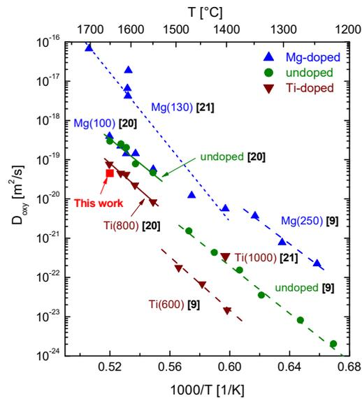
Fig. 4 Impact of Mg or Ti doping on the self-diffusion of oxygen in single crystalline  $\alpha\text{-Al}_2\text{O}_3$ . Data from Lagerlöf et al. [9], Reddy & Cooper [20], Haneda & Monty [21]. Full green circles: nominally undoped; triangles pointing upwards: Mg-doped; triangles pointing downwards: Ti-doped; numbers in brackets: dopant concentrations in wt ppm or at. ppm (see text); red square: this work (mean value of the oxygen diffusion coefficients shown in Fig. 2).
