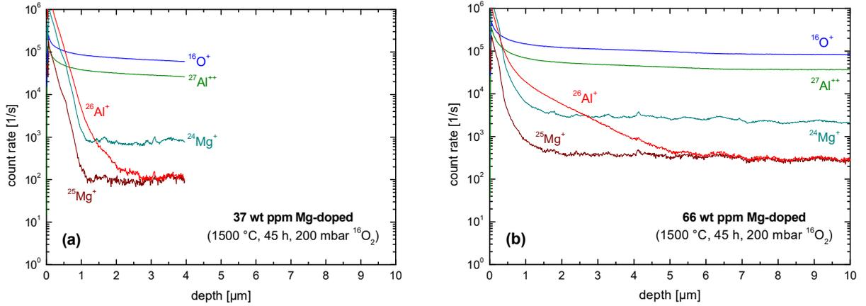
Fig. 3 SIMS raw data of  $^{26}\text{Al}$  depth profiles in simultaneously annealed Mg-doped samples at 1500 °C, 45 h in 200 mbar  $^{16}\text{O}_2$ . (a) 37 wt ppm Mg-doped, (b) 66 wt ppm Mg-doped.
