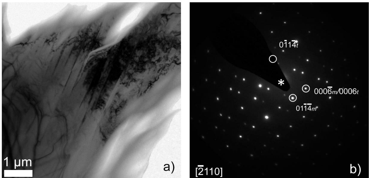
Fig. 1 (a) Sample area of the 66 ppm Mg-doped sample depicting polysynthetic basal twinning. (b) SAED pattern of the area in (a) with beam along the corundum a-axis.
