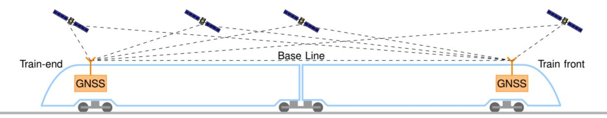
A GNSS receiver measures pseudorange, Doppler and carrier phase to multiple satellites in view.
