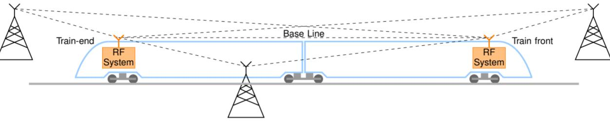
• Measurements: Ranges (Round-trip Delays), Doppler
