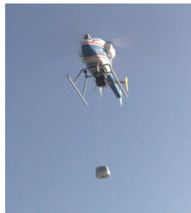
Fig. 6 Portable winch device being lowered
