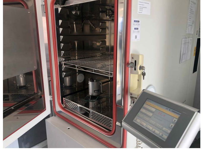
Fig. 5. Ambient temperature test carried out in a weathering chamber.
