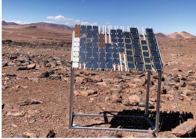
**FIGURE 2.** Clamping structure of the reflectors in Chajnantor (Chile)
