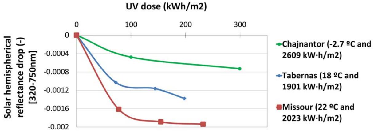
FIGURE 4. Solar hemispherical reflectance drop [320-750 nm] in function on the UV dose received for reflectors exposed in Chajnantor, Tabernas, Missouri
