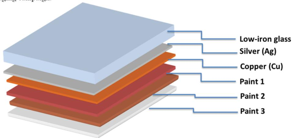
FIGURE 1. Scheme of a silvered-glass reflector
