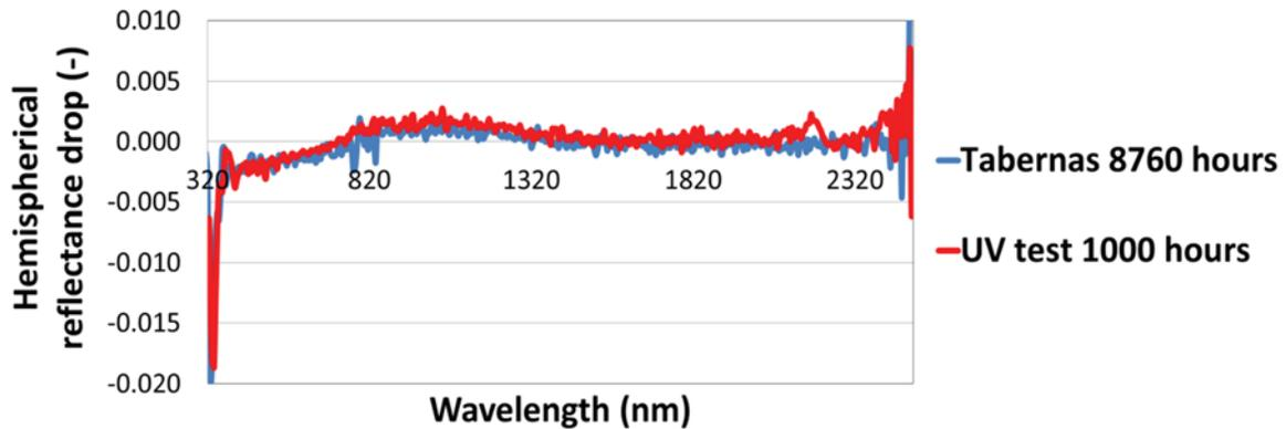
FIGURE 3. Hemispherical reflectance drop [320-2500 nm] after 8760 h of outdoor exposure in Tabernas (Spain) and 1000 h of UV test
