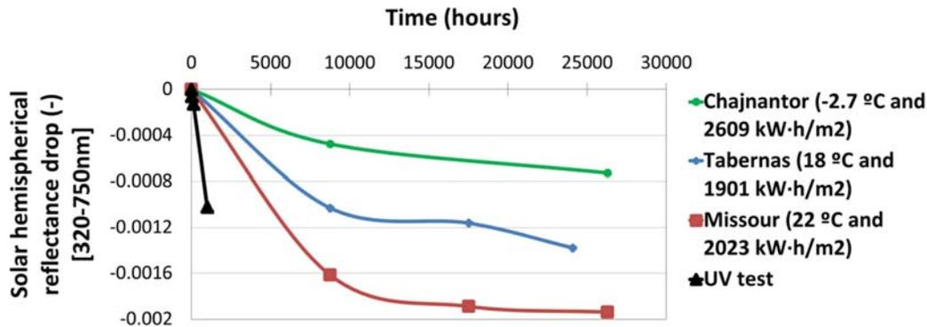
FIGURE 5. Solar hemispherical reflectance drop [320-750 nm] in function on the exposure time for reflectors located in Chajnantor, Tabernas, Missouri and submitted to accelerating aging conditions in a UV test
