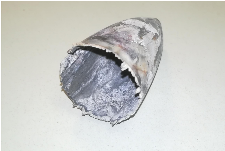
Fig. 11 Nozzle clogging of run 023-V38-END (conversion time).
