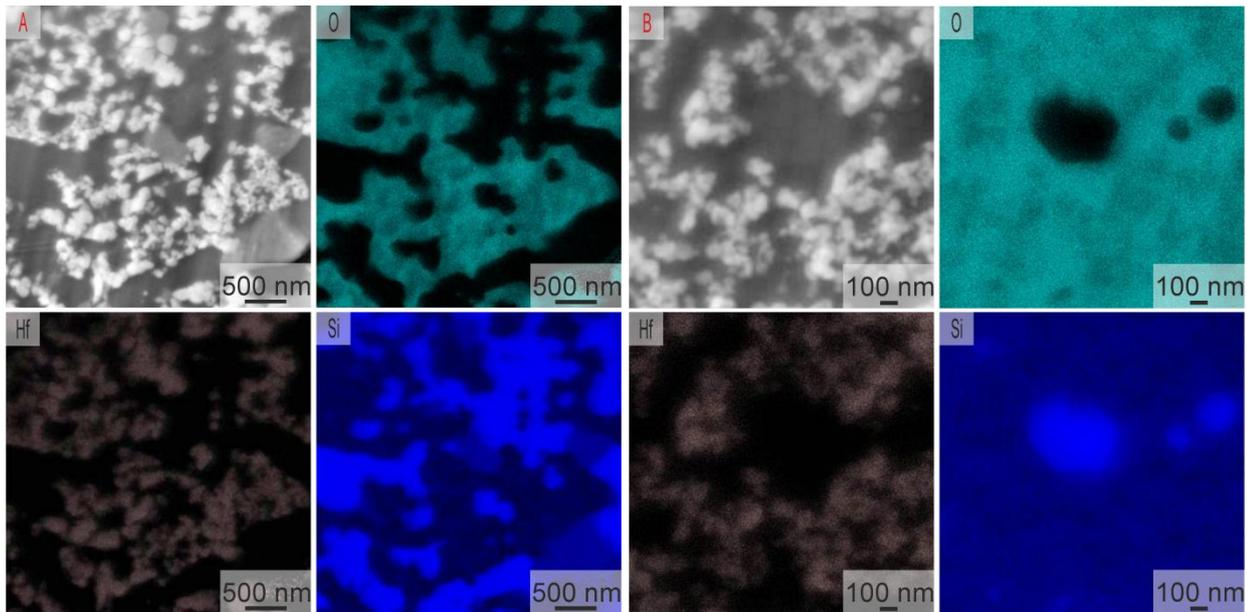
Fig. 12. TEM/EDS mapping of the 500 h tested 60 mol% HfO<sub>2</sub>-doped BC; left: close to the substrate (A); right: close to the surface (B).
