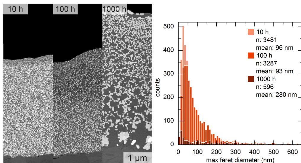
Fig. 7. Left: EsB-SEM cross section images of the 60 mol% HfO<sub>2</sub>-doped Si-BC FCT for 10 h, 100 h and 1000 h; right: histogram of the max feret diameter distribution for the HfO<sub>2</sub>/HfSiO<sub>4</sub> particles at the different testing times. The histogram shows only the first 90 % of the max feret diameter due to a clearer visualization but all particles are considered in the statistics.
