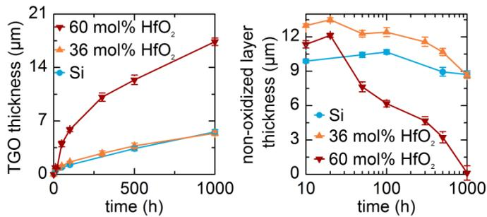
Fig. 14. Left: increase in TGO thickness over the furnace cycle testing time at 1523 K; right: decrease in non-oxidized layer thickness over the FCT time at 1523 K.
