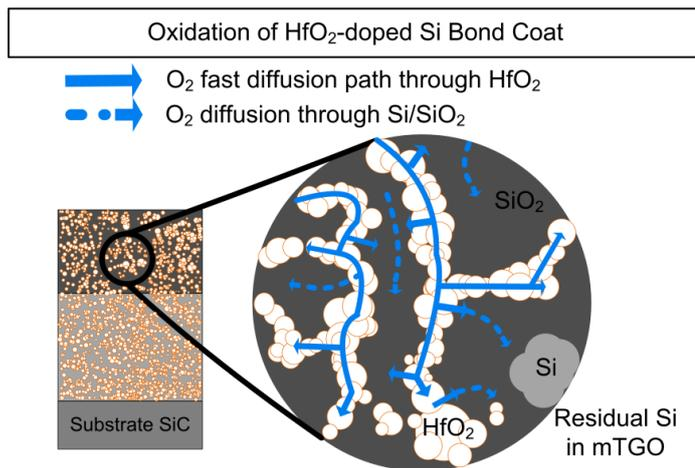
Fig. 16. Schematic of the oxidation of the high hafnia-doped coatings by fast diffusion paths through or along connected hafnia particles and slower diffusion through Si/SiO<sub>2</sub>.
