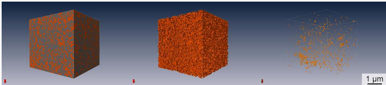
Fig. 9. 3D reconstruction of the 60 mol% HfO<sub>2</sub>-doped Si-BC FCT for 100 h; HfO<sub>2</sub> particles in orange; Si/SiO<sub>2</sub>/pores in grey; left: whole reconstruction; middle: only HfO<sub>2</sub> particles; right: free, unconnected HfO<sub>2</sub> particles.
