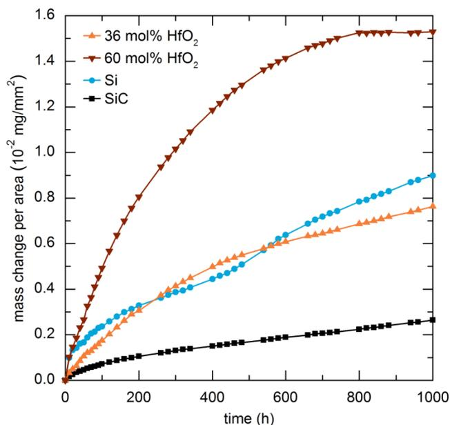
Fig. 13. Mass change per area curves over furnace cycle testing time at 1523 K.
