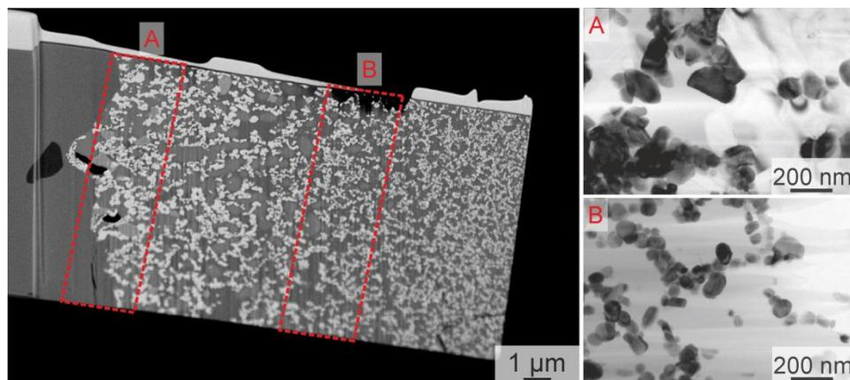
Fig. 11. Left: TEM lamella of the 500 h FCT 60 mol% HfO<sub>2</sub>-doped BC with two red framed areas representing the regions of interest. Right: representative TEM bright-field images showing the hafnia precipitates of the 500 h tested 60 mol% HfO<sub>2</sub>-doped Si-BC; A: close to the substrate; B: close to the surface.
