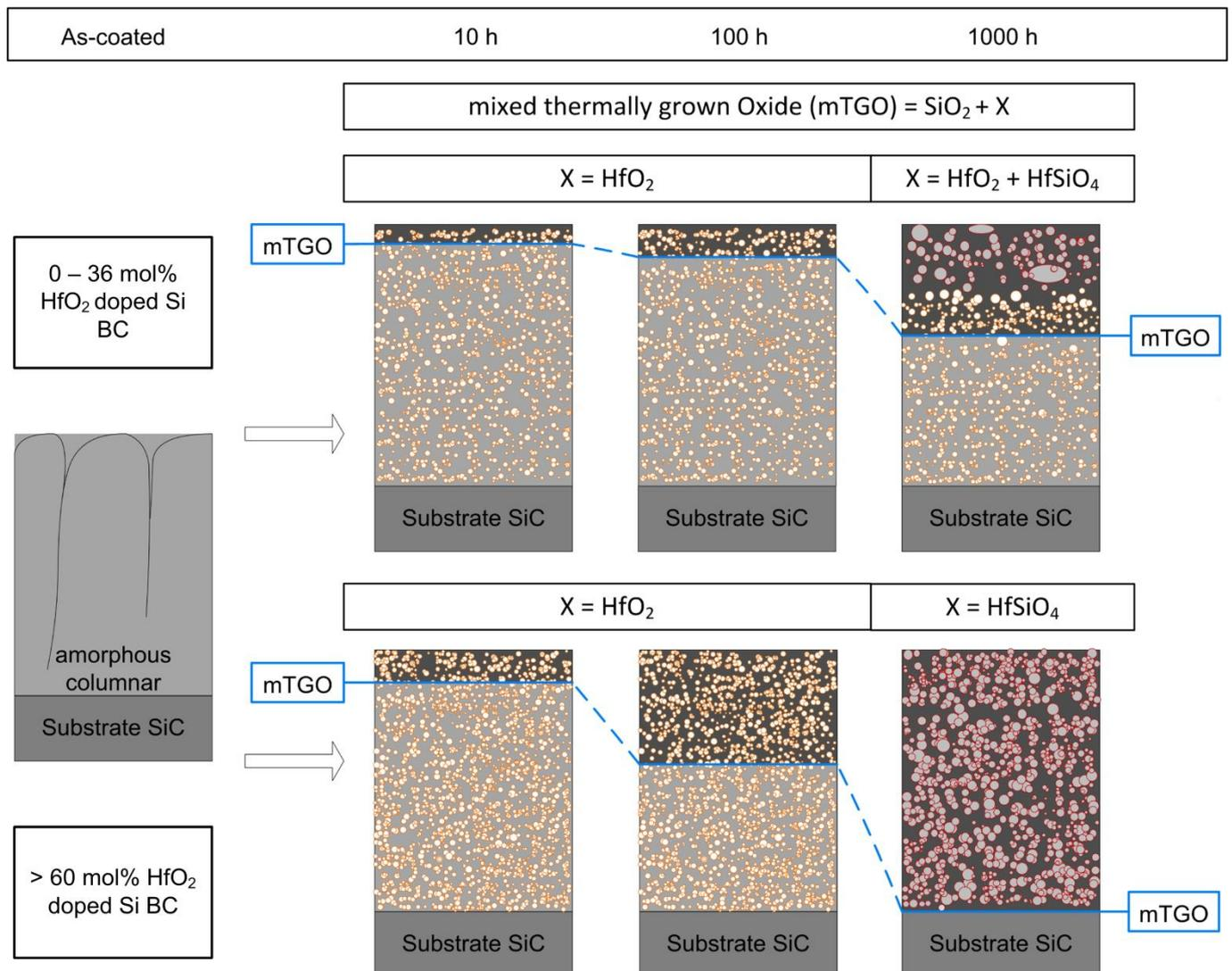
Fig. 17. Schematic evolution of hafnia-doped Si-BCs during various FCT stages showing the increase of the mTGO and the phase formation. The blue line symbolises the interface between mTGO and the remaining BC.
