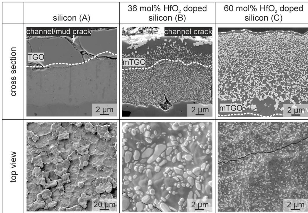
Fig. 4. BC and TGO/mTGO formed on top after 1000 h of FCT testing at 1523 K showing some crack formation after 1000 h of FCT testing at 1523 K; A: silicon showing partial TGO spallation and heavy cracking; B: 36 mol% HfO<sub>2</sub>-doped silicon showing some channel cracks; C: 60 mol% HfO<sub>2</sub>-doped silicon showing least vertical cracking.
