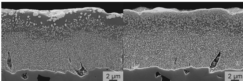
Fig. 5. Overview of the 36 mol% HfO<sub>2</sub>-doped silicon BC after 1000 h of FCT testing at 1523 K showing variations in HfO<sub>2</sub> precipitate size and distribution along the coating.
