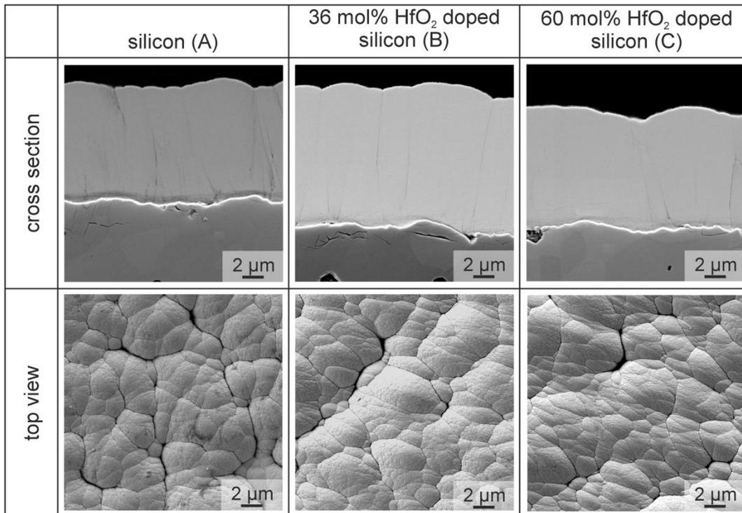
Fig. 1. BC in the as-coated state showing a columnar structure in cross section and cauliflower appearance of the columns in top view; A: silicon; B: 36 mol% HfO<sub>2</sub>-doped silicon; C: 60 mol% HfO<sub>2</sub>-doped silicon.
