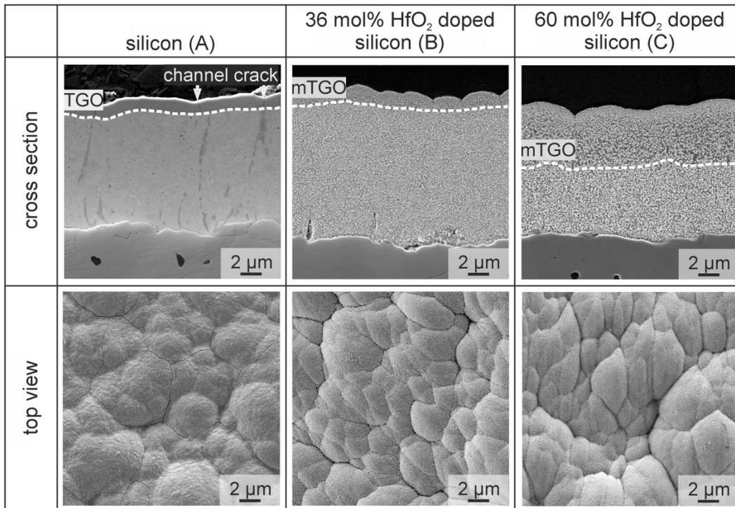
Fig. 3. BC and TGO/mTGO formed on top after 100 h of FCT testing at 1523 K; A: TGO develops channel cracking; B: homogeneously distributed HfO<sub>2</sub> and thin mTGO layer; C: homogeneously distributed HfO<sub>2</sub> and thick mTGO layer.
