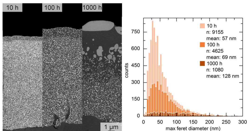
Fig. 6. Left: EsB-SEM cross section images of the 36 mol% HfO<sub>2</sub>-doped Si-BC FCT for 10 h, 100 h and 1000 h; right: histogram of the max feret diameter distribution for the HfO<sub>2</sub>/HfSiO<sub>4</sub> particles at the different testing times. The histogram shows only the first 90 % of the max feret diameter for a clearer visualization but all particles are considered in the statistics.
