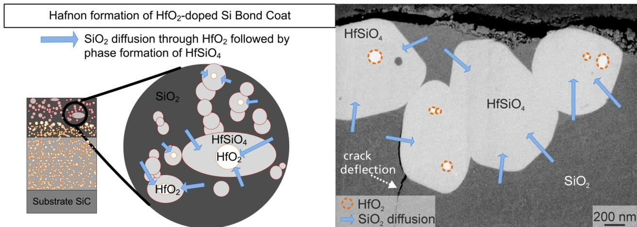
Fig. 15. Schematics of reaction between  $\text{HfO}_2$ ,  $\text{SiO}_2$  and  $\text{HfSiO}_4$  phase formation by mostly diffusion of  $\text{SiO}_2$  into  $\text{HfO}_2$  (left) and EsB picture of the 36 mol%  $\text{HfO}_2$ -doped BC (right). The bright particles visible in EsB picture have been circled and evidently they are rich in hafnium.
