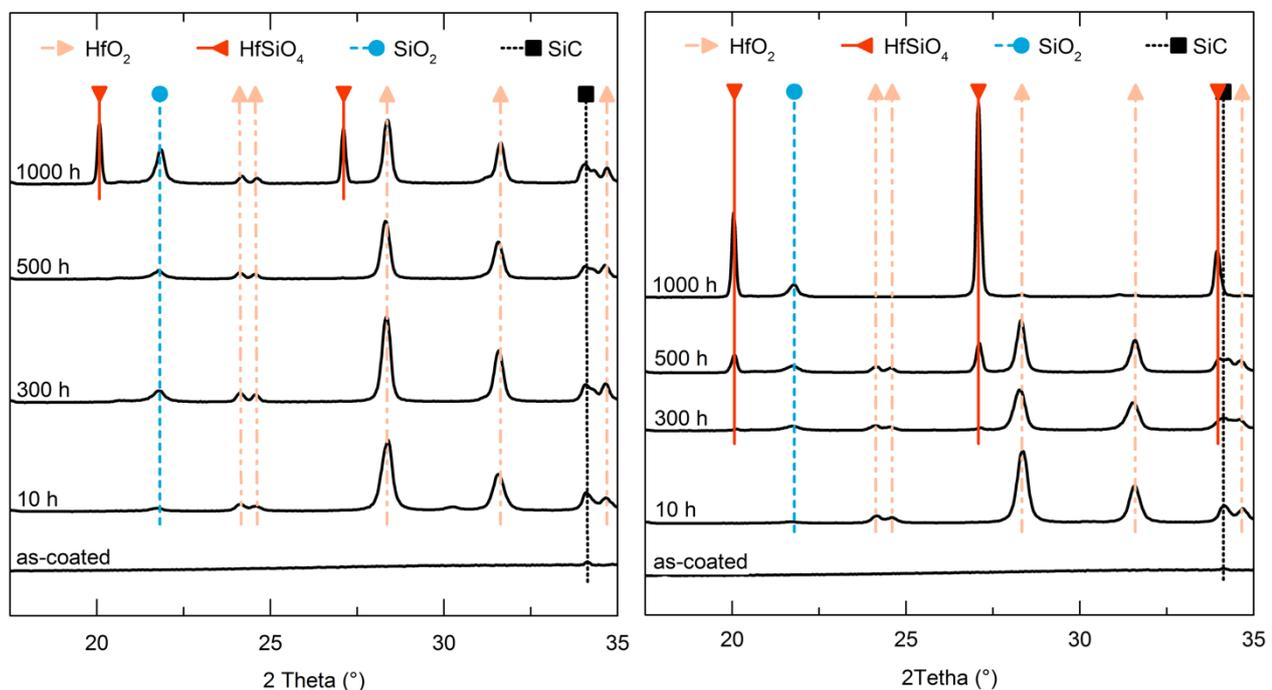
Fig. 10. Relevant part of the XRD scan from 15° - 35° 2θ of HfO<sub>2</sub>-doped Si-BC for different testing times; left: 36 mol% HfO<sub>2</sub>; right: 60 mol% HfO<sub>2</sub>.
