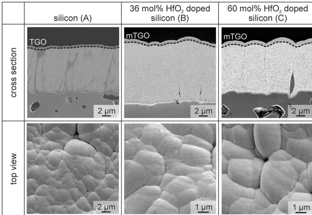
Fig. 2. BC and TGO/mTGO formed on top after 10 h of FCT testing at 1523 K; A: silicon; B: 36 mol% HfO<sub>2</sub>-doped silicon; C: 60 mol% HfO<sub>2</sub>-doped silicon.
