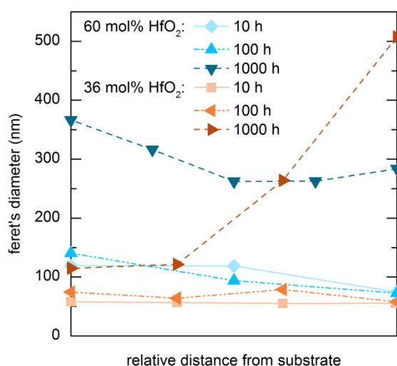
Fig. 8. Development of mean feret diameter in relative distance to the SiC substrate of the HfO<sub>2</sub>/HfSiO<sub>4</sub> particles in the HfO<sub>2</sub>-doped Si-BC FCT for 10 h, 100 h and 1000 h.
