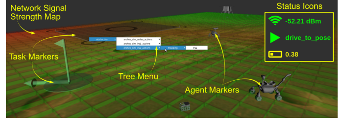
Fig. 5: Screenshot of the 3D GUI and status icons (per robot) of the ROSMC high-level mission control framework.
