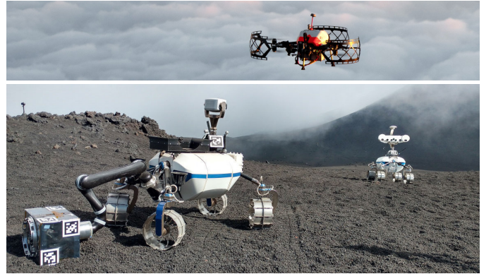
Fig. 1: Our Lightweight Rover Units (LRUs) [5] and drone ARDEA [7] test their skills for autonomous navigation, exploration, and sampling at a Moon-analogue site on Mt. Etna.
