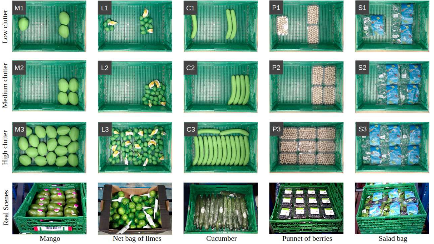
Fig. 3. First three rows: Protocol scenarios sorted by object type and amount of clutter. Last row: Real placement scenes.
