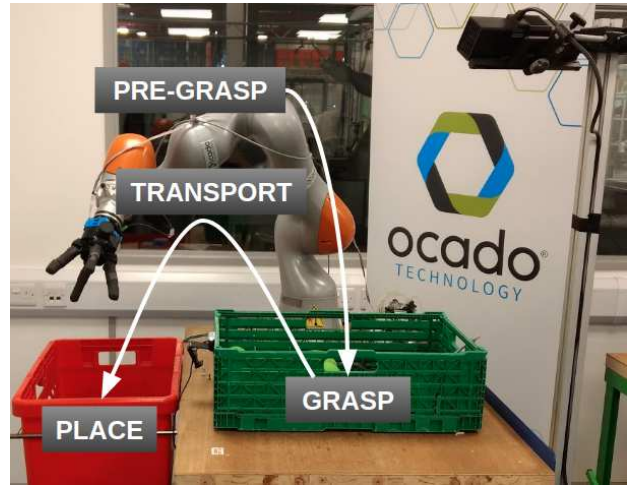
Fig. 1. Phases considered for benchmarking pick-and-place tasks.
