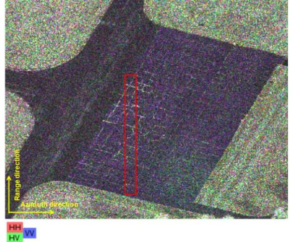
Fig. 7. RGB composite generated from F-SAR intensity images
