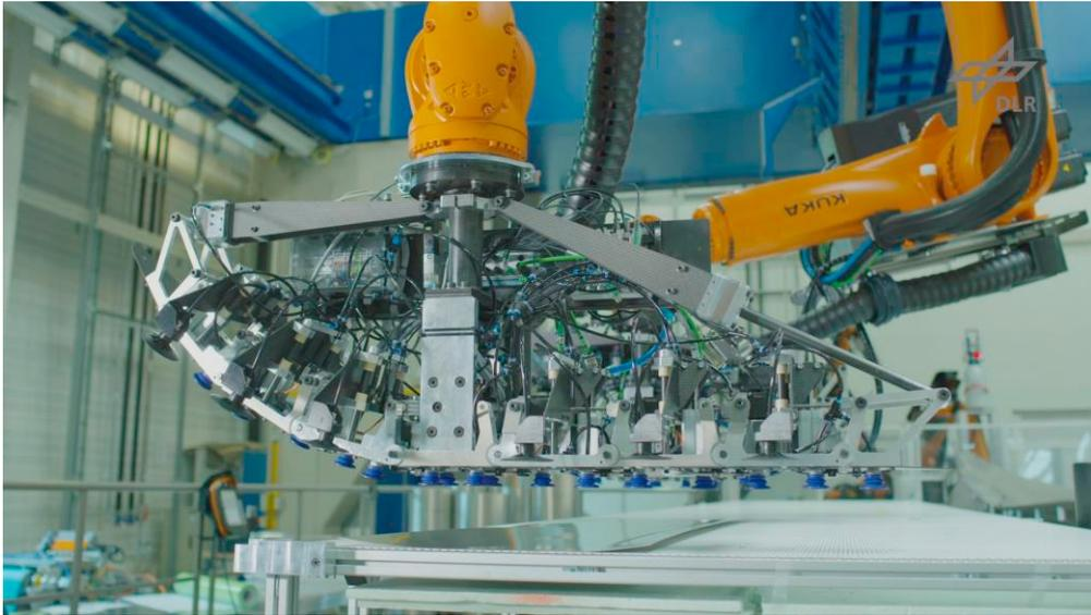
Figure 1: One of the grippers with one arm fully curved (left) and one arm straightened (right)
