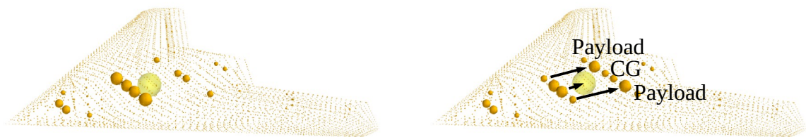
Figure 5.13: A rearward shift of payload creates a unstable configuration. Left: M11, Right: M11b
