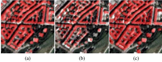
Fig. 3. Comparison of results generated by U-Net structure with different depths. (a) Depth ( d = 5 ); (b) Depth ( d = 8 ); (c) Ground truth.
