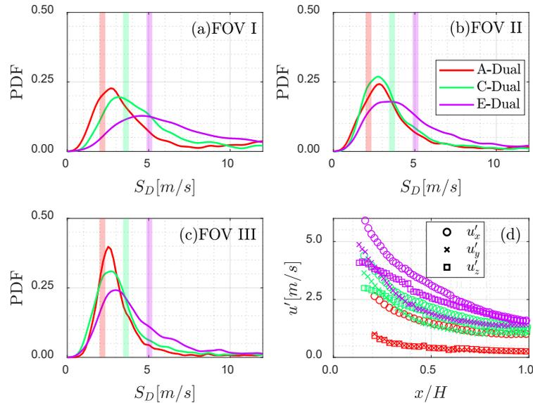
**Figure 12: PDFs of reactant pocket displacement speeds: (a) FOV I, (b) FOV II, and (c) FOV III. Vertical colored lines represent  $S_D = u'$ : 2.2 m/s for A-Dual, 3.6 m/s for C-Dual, and 5.0 m/s for E-Dual at the burner exit location. (d) Turbulence intensities along  $\bar{c} = 0.5$  as functions of downstream distance for cases Dual-A, C, and E**
