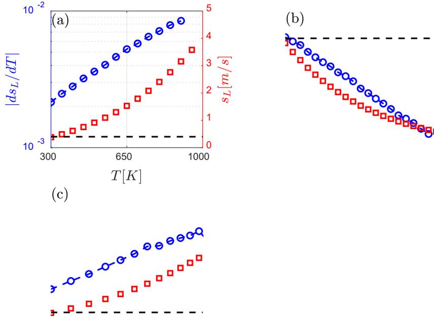
**Figure 15: Laminar flame speed variations due to: (a) preheating of reactants, (b) addition of diluents, and (c) addition of hot combustion products. (d) Equilibrium temperatures as a function of diluent addition. Dashes horizontal lines in sub-figures (a)-(c):  $s_L=0.4$  m/s**
