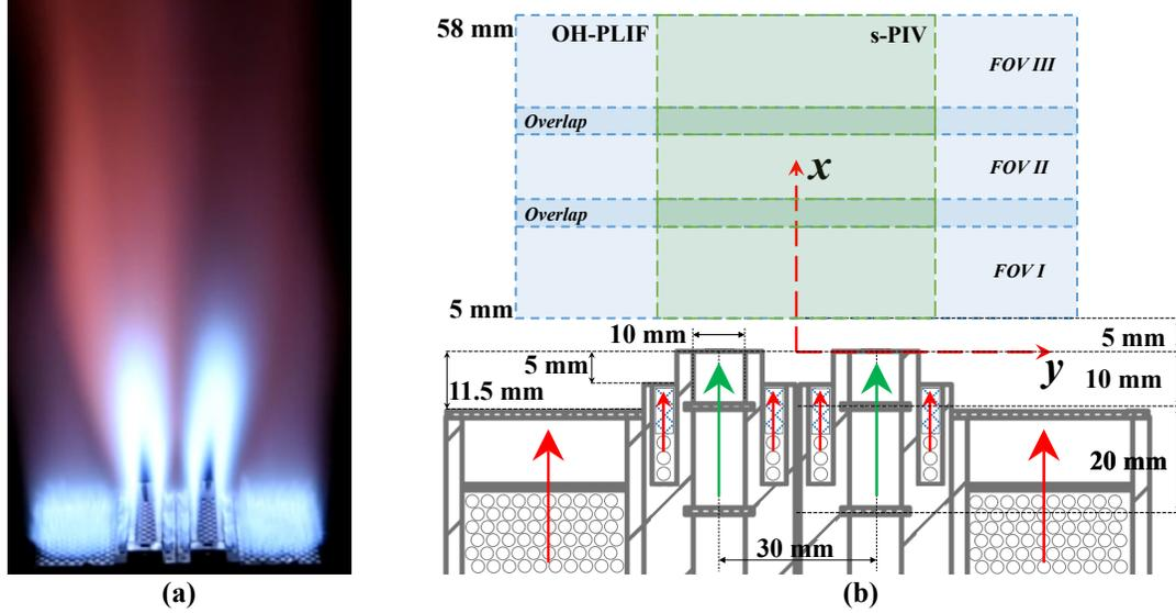
**Figure 1: (a) Photograph of dual burner experiment in operation with all pilot flames. (b) Fields-of-views (FOVs) for optical measurements; the red arrows represent the flow path for the pilot flame premixed gases and the green arrows represent the flow path for the main flame premixed gases**
