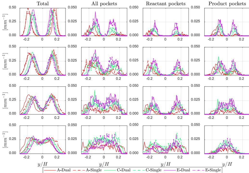
**Figure 6: Horizontal slices of flame surface density contributions at various downstream locations: (a)  $x/H=0.25$ , (b)  $x/H=0.5$ , (c)  $x/H=0.75$ , and (d)  $x/H=1$ . For comparisons between single- and dual-flames, the y-axis is adjusted to the left burner centerline in dual-flames cases. For clarity, every fifth data point is plotted here**
