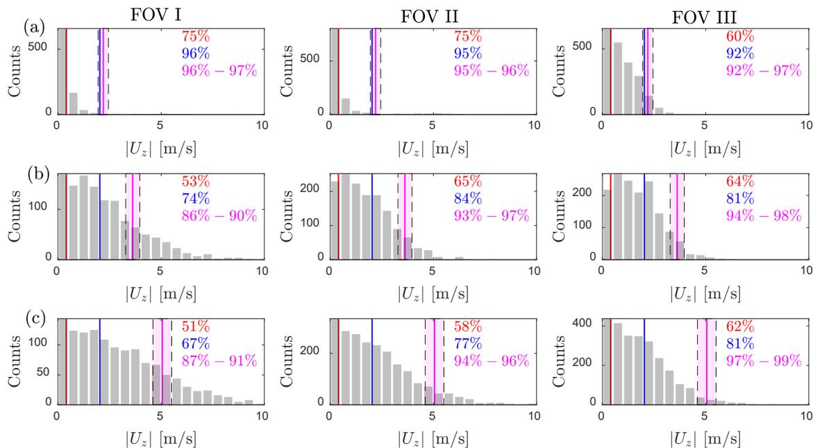
**Figure 14: Histograms of the magnitudes of averaged out-of-plane instantaneous velocity within product pocket contours in (a) Dual-A, (b) Dual-C, and (c) Dual-E. Red-vertical lines:  $s_L$ , blue-vertical lines:  $s_{L,max}$ , and magenta-vertical lines:  $S_T \pm \delta S_T$**
