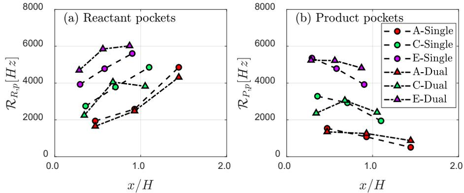
**Figure 8: Frequency of pocket formations in [Hz] for: (a) reactant pockets, (b) product pockets**
