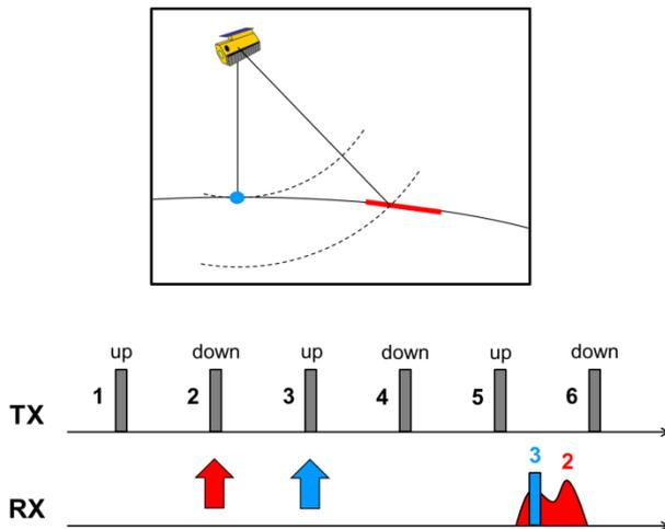
**Figure 3** Waveform variation scheme, and superposition of nadir echo (blue) and useful signal (red) in the received signal.
