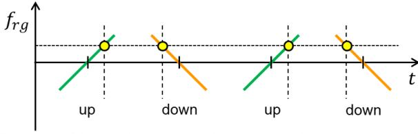
**Figure 5** Non-uniform sampling caused by using up and down chirp alternation for waveform variation.
