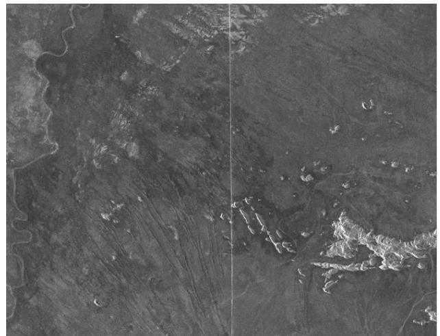
**Figure 1** TerraSAR-X image over Australia as an example of nadir echo in a SAR image, where the horizontal and vertical axes represent slant range and azimuth, respectively. The nadir echo, a bright vertical line, appears in the middle of the image.
