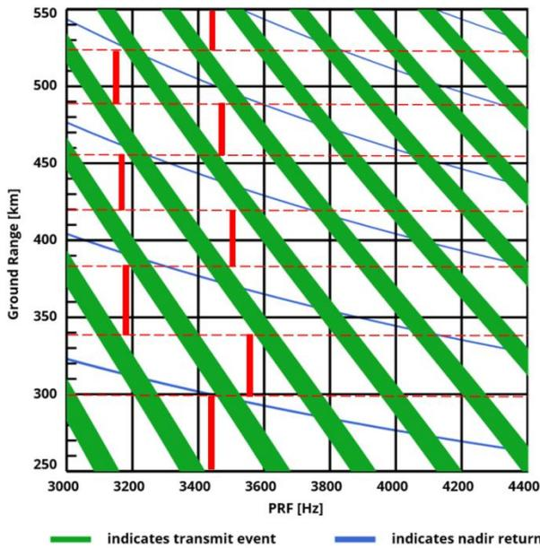
**Figure 2** Timing diagram for PRF selection of conventional SAR. The green and blue areas are transmit and nadir interferences, respectively, while the red lines indicate possible swaths that avoid transmit and nadir interferences.
