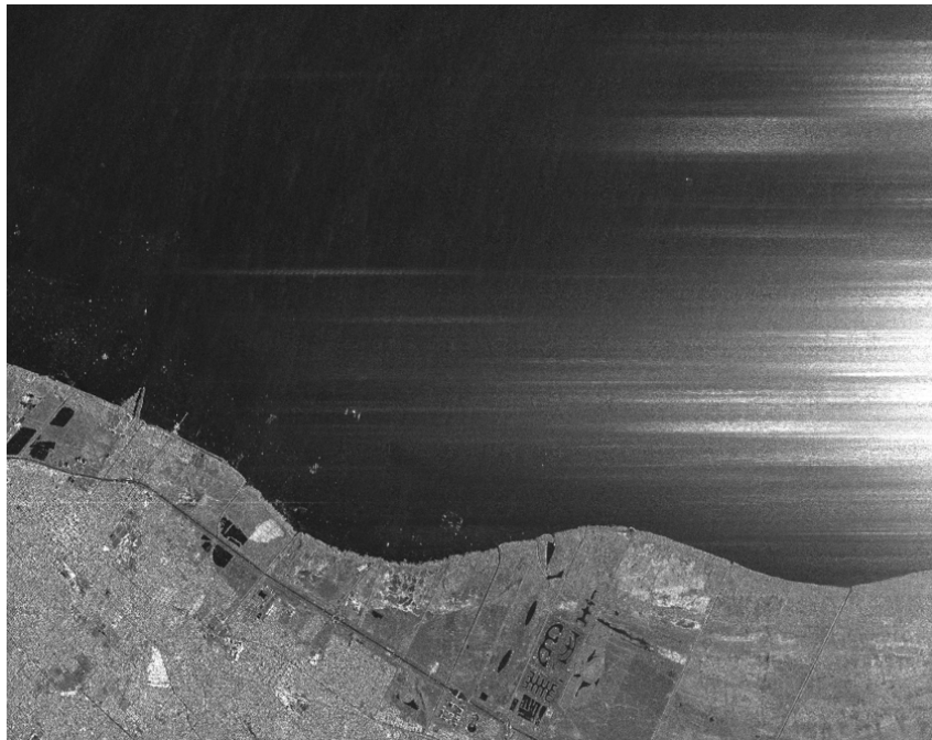
FIGURE 4.14 – Focused image of the off-nominal experimental Stripmap acquisition over Buenos Aires, Argentina.
