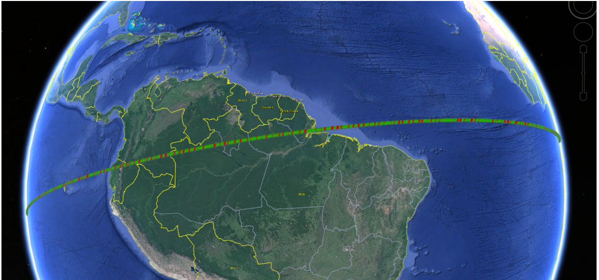
FIGURE 5.5 – Available targets at latitude zero are depicted in green, whereas areas which are not accessible with the concurrent imaging technique are depicted in red. A symmetrical 30 km/5 km SM/ST overlapping scenario is considered. Scene center incidence angle must be within the data collection range.
