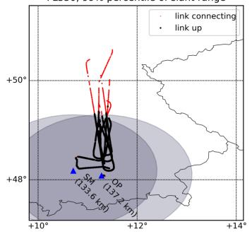
measured range at 40 dBM TX power is 133.6/137.2 km for SM/OP groundstation
