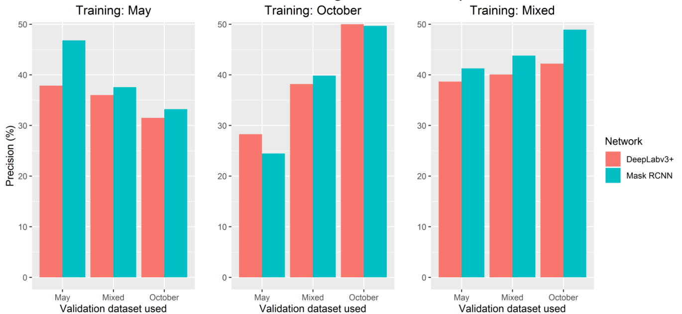
Figure 22 Precision scores for both DeepLab and Mask R-CNN using three different seasonal datasets (May, October, and a mixture of the two) split into training and validation sets. Networks were trained on one of the three datasets and subsequently assessed using each of the three validation datasets.
