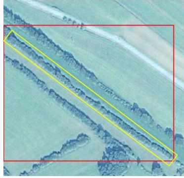
Figure 31 Shows an anchor bounding box without (red) and with (yellow) rotation for a single hedgerow.
