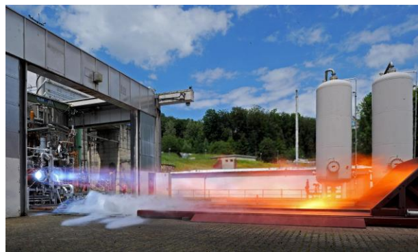
Fig. 20. Test Facility P3.2 during a methane development thrust chamber hotrun
