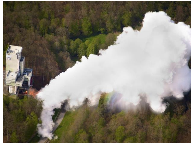
Fig. 23. Exhaust gas and cooling water clouds during a P5 hot-fire test
