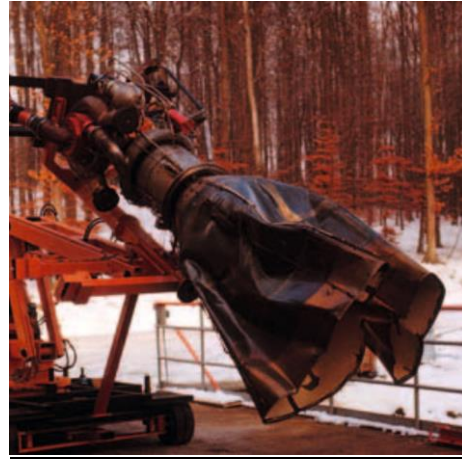
Fig. 10. Viking failures at Test Facility P4.2
