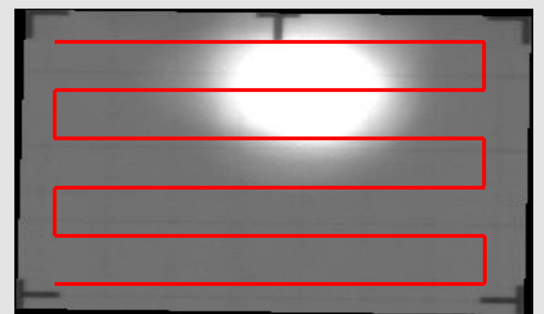
Pic 4: Movement of the Heliostat focal point over the target. The "Neander"-walk would cover the whole Target and will output more Data per calibration. Also a random-walk is conceivable
