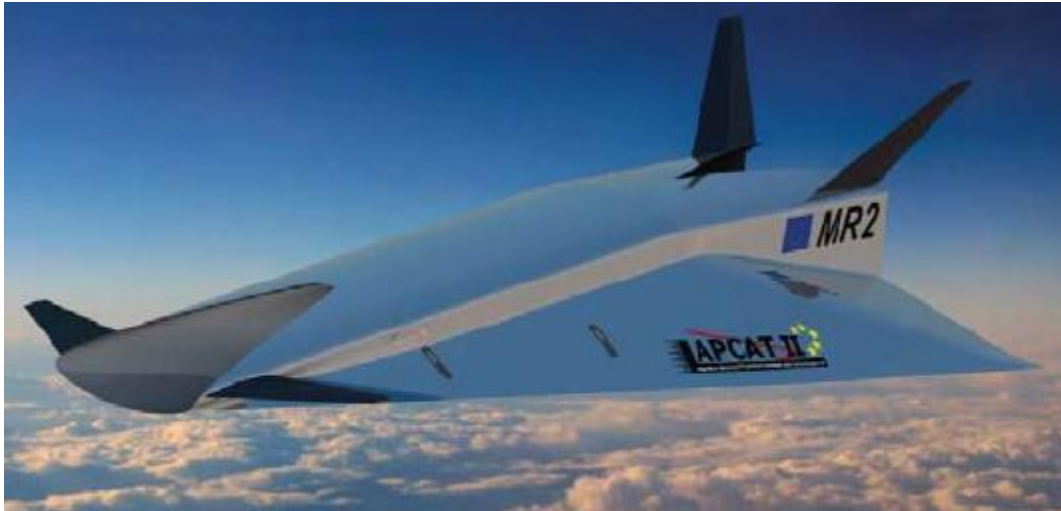
Figure 1: LAPCAT MR2.4, the aircraft design basis for STRATOFLY
