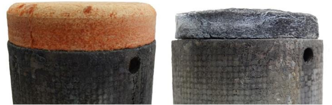
Figure 9: ZURAM ® -K sample V2 #4 before (left) and after test (right) in L2K facility (heat flux: 0.91 MW/m 2 , test duration: 62 s)
