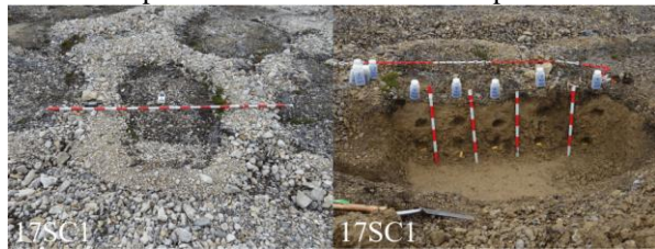
Fig. 2: Sorted stone circle 17SC1 on Svalbard. View before trenching (left) and the sampled cross section of the circle (right).
