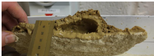
Figure 2: Details of the exposed inner structure of the two different frozen mud flows in which the liquid core was still present. Note the bubbles trapped in ice near the ruler.
