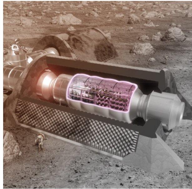
Fig. 2: Space greenhouse design based on lessons learned from EDEN ISS MTF in Antarctica, credit: EDEN ISS Consortium, visualisation: LIQUIFER Systems Group, 2019
