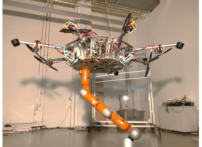
Fig. 1. A prototype of the active cable-suspended aerial manipulator SAM.
