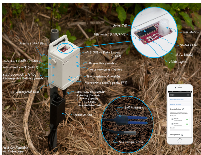
Fig. 1: Sensors are fully autonomous nodes with wireless communication and solar energy harvesting for collecting data from ground and atmospheric probes.
