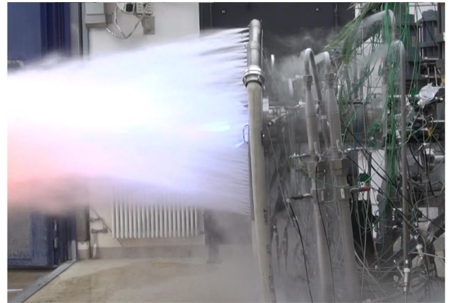
Fig. 6 Picture of the combustion chamber in the test cell and the protecting water shield during a hot run.
