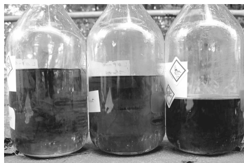
Figure 2. Prepared LMP-103S samples contaminated with metal ions.
