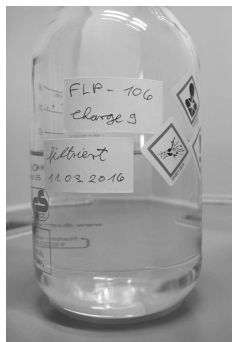
Figure 1. Prepared ADN-based monopropellant FLP-106.
