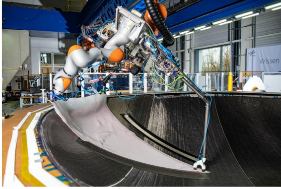
(a) Fixing of auxiliary package with Multi-kinematic gripper
