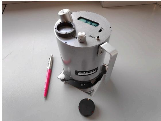
**Figure 2.** Portable specular reflectometer 15R-USB by Devices and Services (D&S).
