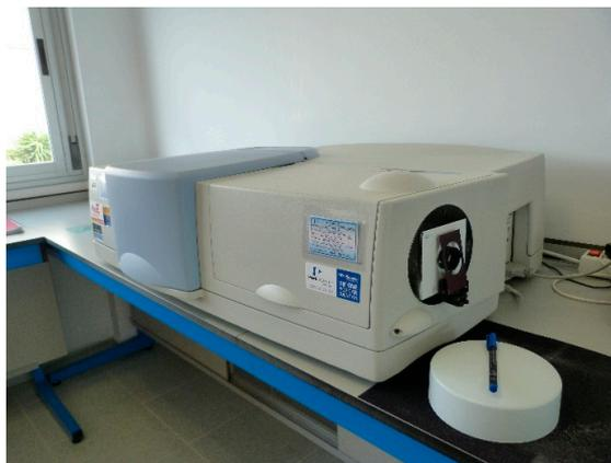
**Figure 3.** Spectrophotometer Lambda 1050 by Perkin Elmer (PE).
