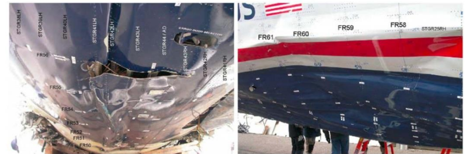
Structural deformation in the rear bottom section of the A320 ditched on the Hudson River [2]
