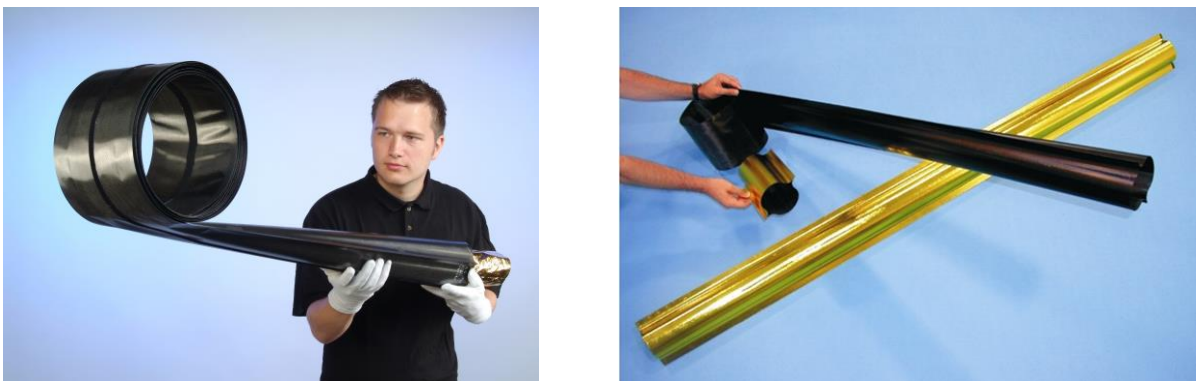
Figure 2: Reelable double omega boom developed by DLR in partly stowed configuration (left) and boom samples with surface coating (right) [Courtesy: DLR].
