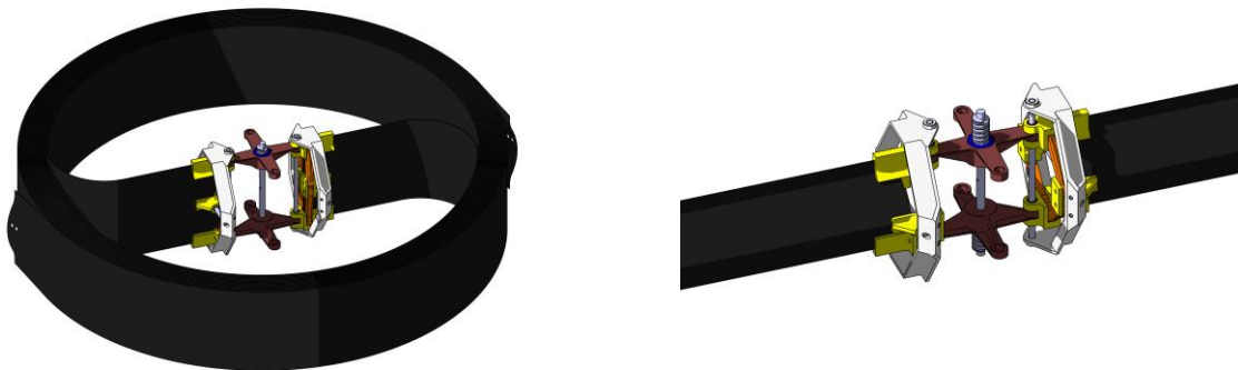
Figure 7: Boom root interface with two of four booms in stowed (left) and deployed configuration (right).
