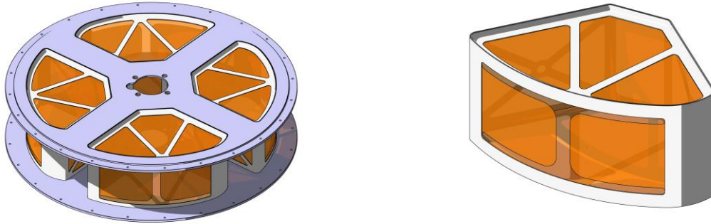
Figure 4: Assembled booms spool composed of two sandwich plates and four sail containers which also form the hub for boom coiling (left); detailed view of a single sail container with framework structure and inner Kapton liner (right).
