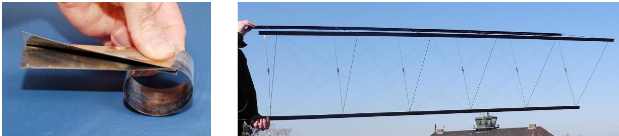
Figure 13: Examples of applicable reelable booms: TRAC (Triangular Rollable and Collapsible) [2] boom for small, meter-class sails (left) and CTT (Collapsible Tape Truss) [11] for hundred-meter class solar sails (right).
