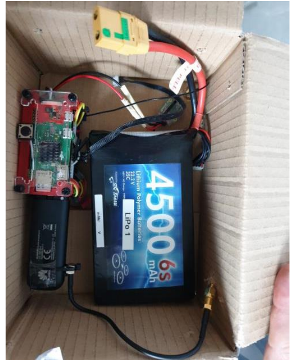
Figure 8 - Air Unit with LiPo battery inside cardboard box
