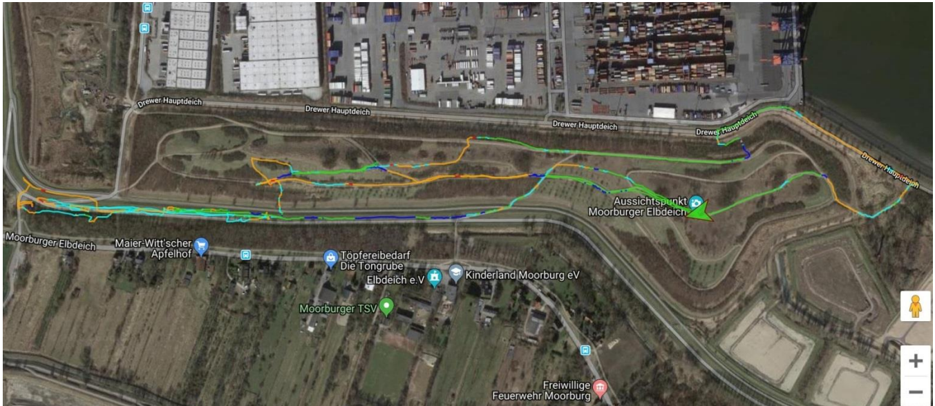
Figure 10 – Connectivity of 868 MHz, 2.4 GHz and LTE link in urban environment
