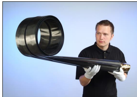
Figure 1: Tubular shell mast with double-omega cross-section developed by DLR that is stowed through reeling.
