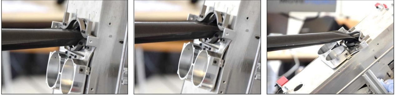
Figure 2: Typical buckling failure mode of a tubular shell mast at the interface towards the deployment mechanism due to insufficient support against shell deformation to the inside [Courtesy of DLR].
