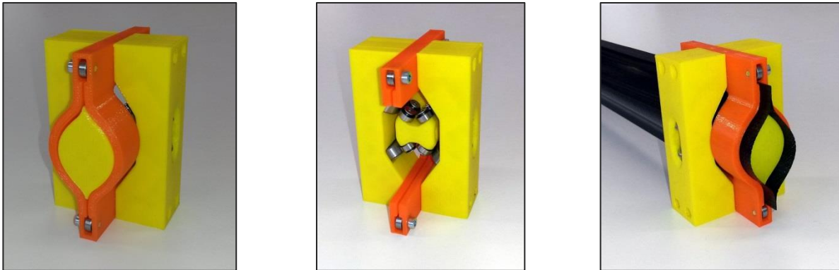
Figure 9: Sliding core interface design with four tilted contact points of the core with enforced form closure.
