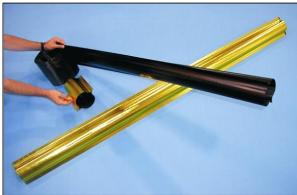
Figure 1: Tubular shell mast with double-omega cross-section developed by DLR that is stowed through reeling.
