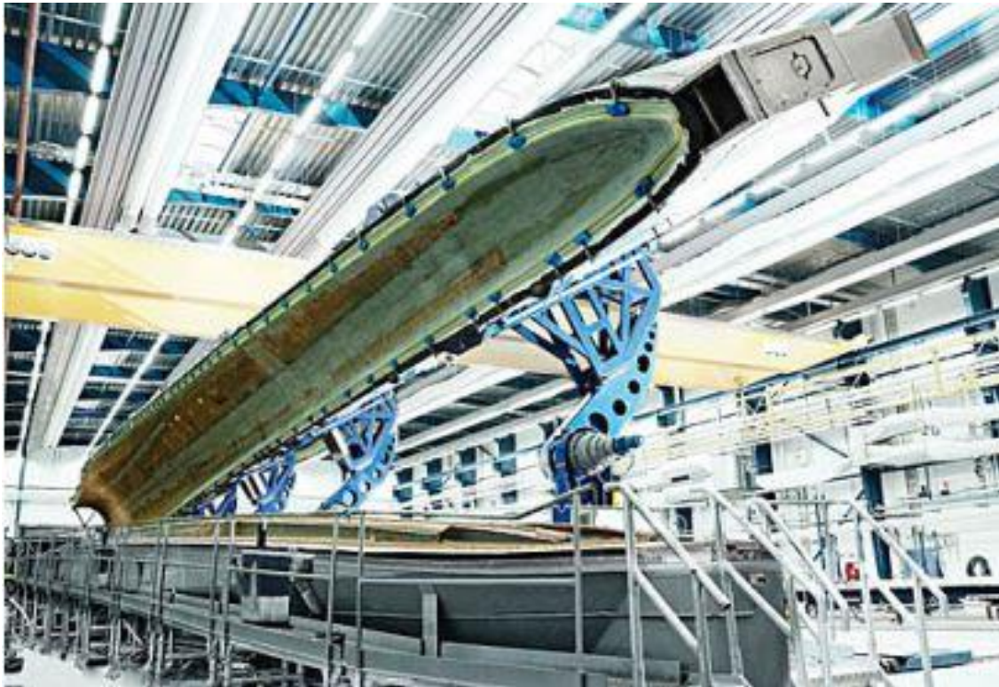
Figure 2-3 Laminating of a Rotor Blade [3]
