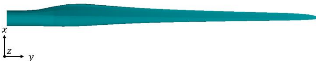
Figure 6-1 Plan View on the FE Model of the Rotor Blade
