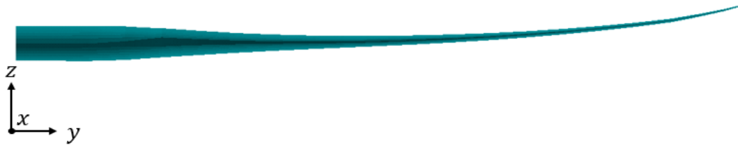
Figure 6-2 Side View on the FE Model of the Rotor Blade
